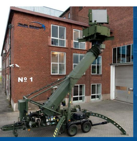
Ability to elevate a radar of up to 2 ton 20 metres up
